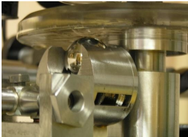
Figure 3, a, b – The contacting tribopair of the indenter and the counterbody in point contact: a – circular contact ( \beta = 1 ); b – elliptical contact ( \beta = 8 )
