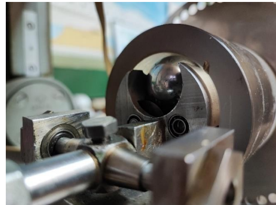
Figure 3, a, b – The contacting tribopair of the indenter and the counterbody in point contact: a – circular contact ( \beta = 1 ); b – elliptical contact ( \beta = 8 )
