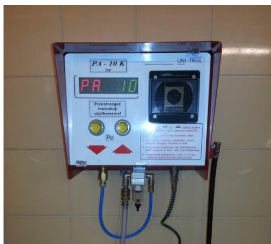
Rysunek 1 – Automat do pompowania kół Unitrol PA – 10K Figure 1 – Unitrol PA – 10K automatic wheel pumping machine
