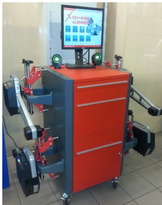
Rysunek 2 – System pomiaru geometrii kół Launch X-631 Figure 2 – Launch X-631 wheel alignment system
